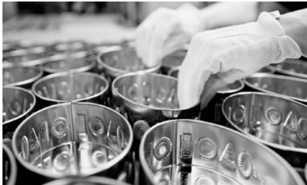
Due to its characteristics, tin plate is an excellent migration barrier, making tin cans a highly popular outer packaging material for the food industry
